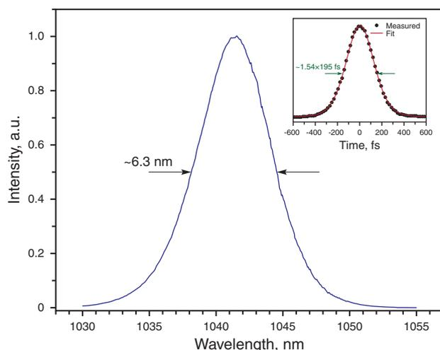
**Figure 3** (online color at [www.lasphys.com](http://www.lasphys.com)) Pulse duration (inset) and corresponding optical spectrum of the femtosecond mode-locked pulses for the case of  $T = 1.6\%$
