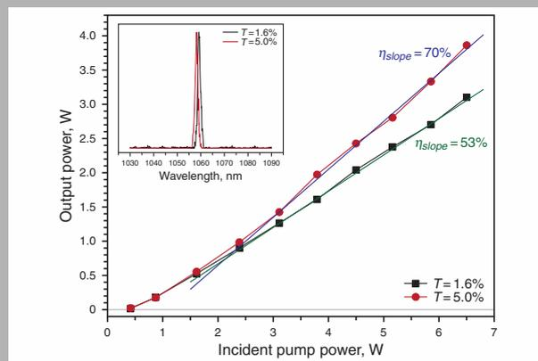
The relationship between the incident pump power and laser output of Yb:LPS laser. The inset shows the corresponding laser wavelengths
