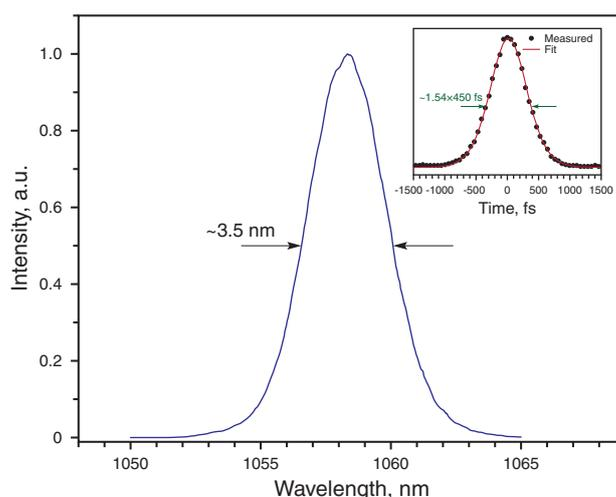
**Figure 4** (online color at [www.lasphys.com](http://www.lasphys.com)) Pulse duration (inset) and corresponding optical spectrum of the femtosecond mode-locked pulses for the case of  $T = 5.0\%$
