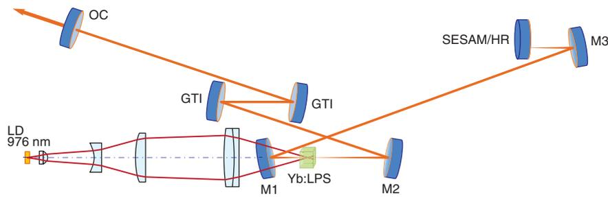
**Figure 1** (online color at [www.lasphys.com](http://www.lasphys.com)) Schematic of the mode-locked Yb:LPS laser setup. M1 – ROC=100 mm HR@1000–1080 nm, M2 – ROC=200 mm HR@1000–1080 nm, M3 – ROC=200 mm HR@1000–1080 nm, and OC – plano output coupler
