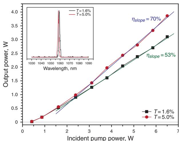
**Figure 2** (online color at [www.lasphys.com](http://www.lasphys.com)) The relationship between the incident pump power and laser output of Yb:LPS laser. The inset shows the corresponding laser wavelengths
