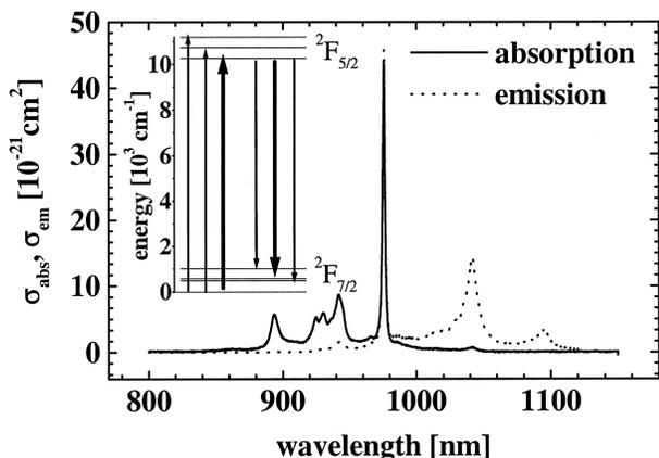
Fig. 1. Absorption and emission spectra of Yb:Sc<sub>2</sub>O<sub>3</sub> and energy-level diagram with the relevant transitions (inset).
