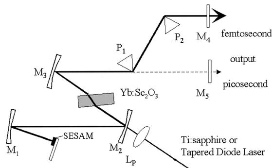
Fig. 2. Schematic of the mode-locked Yb:Sc<sub>2</sub>O<sub>3</sub> laser: M<sub>1</sub>, focusing mirror (RC, 10–15 cm); M<sub>2</sub>, M<sub>3</sub>, folding mirrors (RC, 10 cm); P<sub>1</sub>, P<sub>2</sub>, SF<sub>6</sub> prisms; M<sub>4</sub>, M<sub>5</sub>, output couplers; L<sub>p</sub>, 6.28-cm focusing lens.
