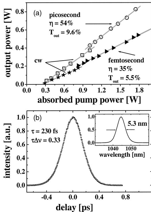
Fig. 3. Performance of the Yb:Sc<sub>2</sub>O<sub>3</sub> mode-locked laser with a Ti:Sa pump source. (a) Output power versus absorbed pump power in the picosecond and femtosecond regimes and below their mode-locking thresholds (cw);  $\eta$ , slope efficiency. (b) Autocorrelation trace and spectrum (inset) in the femtosecond regime.
