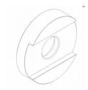
**Mount:** gold-plated copper ring with: 12.7 mm outer diameter
