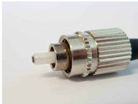
SAM chip on FC/PC connector end face
