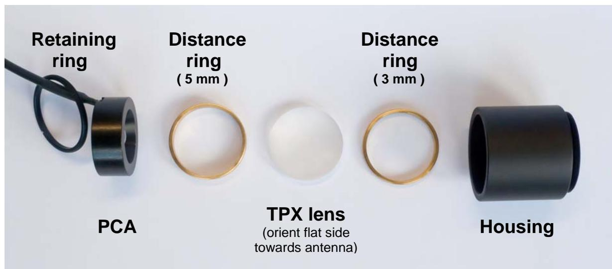
**Fig. 5: Order of components of CTL-D25mm**
