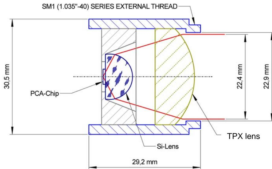
Fig. 3: Schematic section view (PCA + Si-lens not included)
