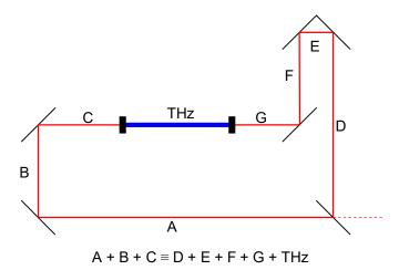
It is advised to meet this condition with the delay stage positioned approximately centred.
