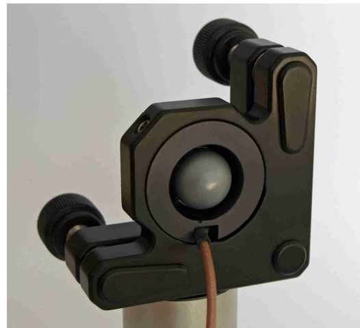
Back view on mounted PCA (THz side)
