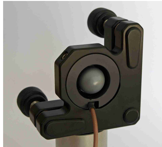
Back view on mounted PCA (THz side)
