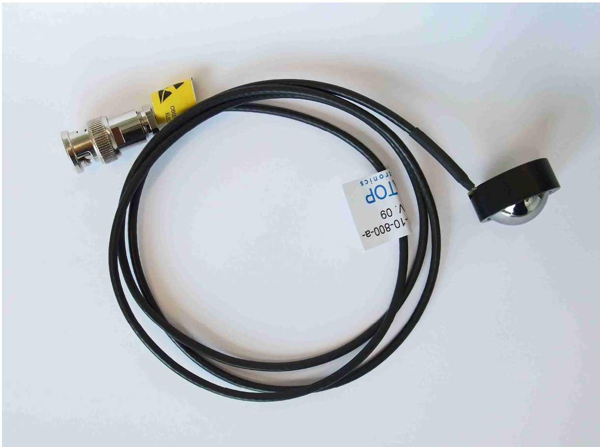
PCA with aspheric silicon lens, coaxial cable RG 178 and BNC connector
