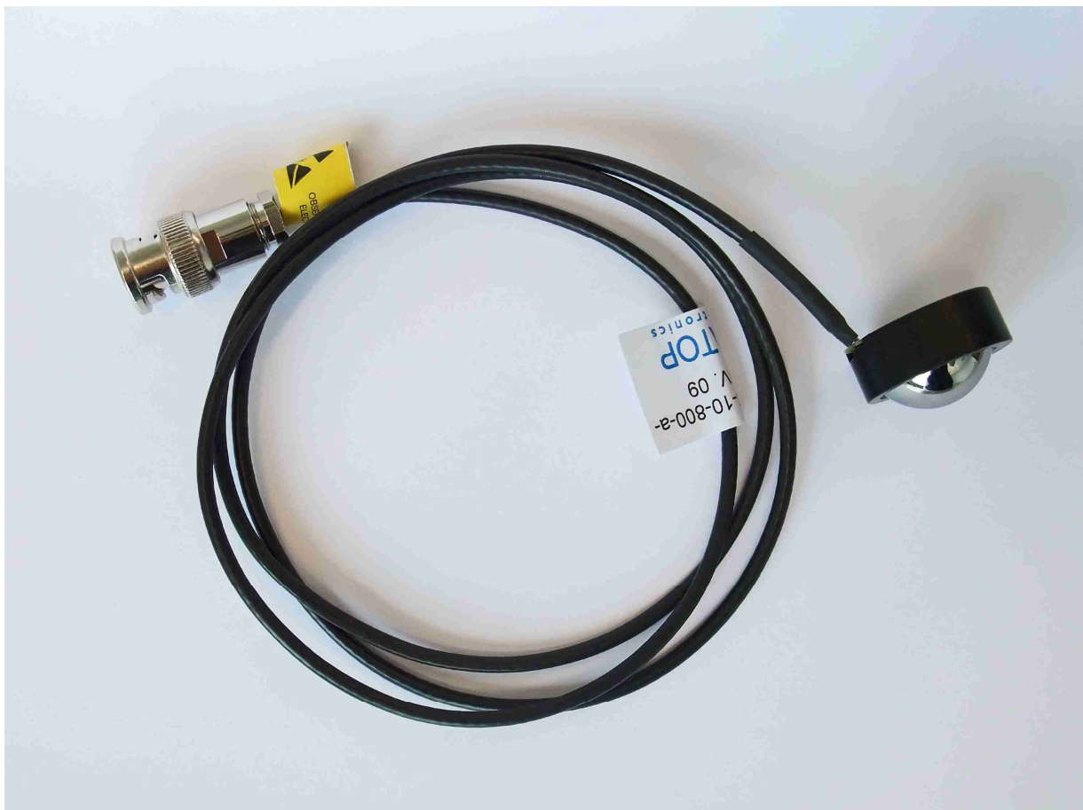
Complete antenna with cable and BNC connector
